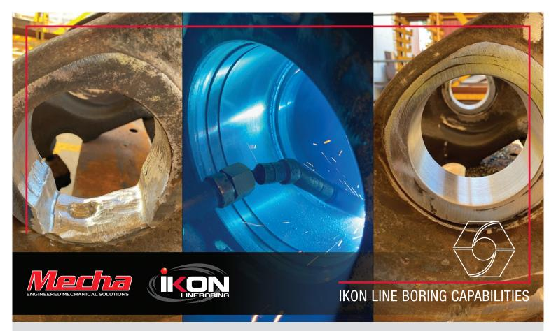
Line boring is an integral engineering practice, seamlessly addressing precision alignment challenges in machinery by precisely machining worn or misaligned bores.
